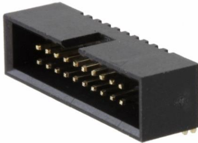
Figure 7: Control Interface connector - Right Angle, 20-position, 2-row, 1.27mm pitch
