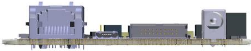
Figure 6: side view of FlashRunner HS Control Unit with LAN connector, USB control port, ATE control connector and power jack.
