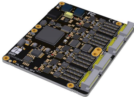
Figure 4: FlashRunner HS GP4 Active Module with right-angle device connectors
