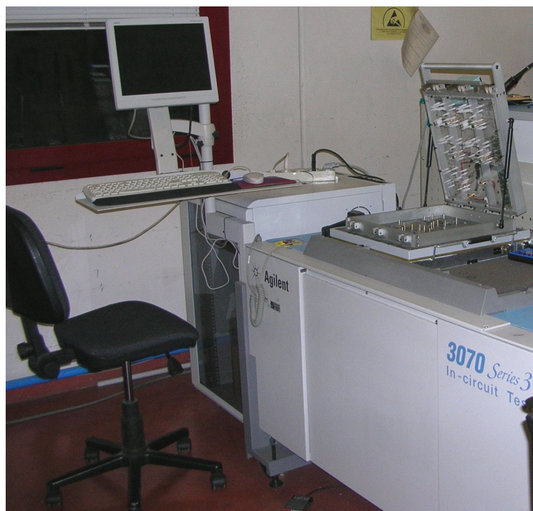
Figure 2. ATE with Manual Fixture
