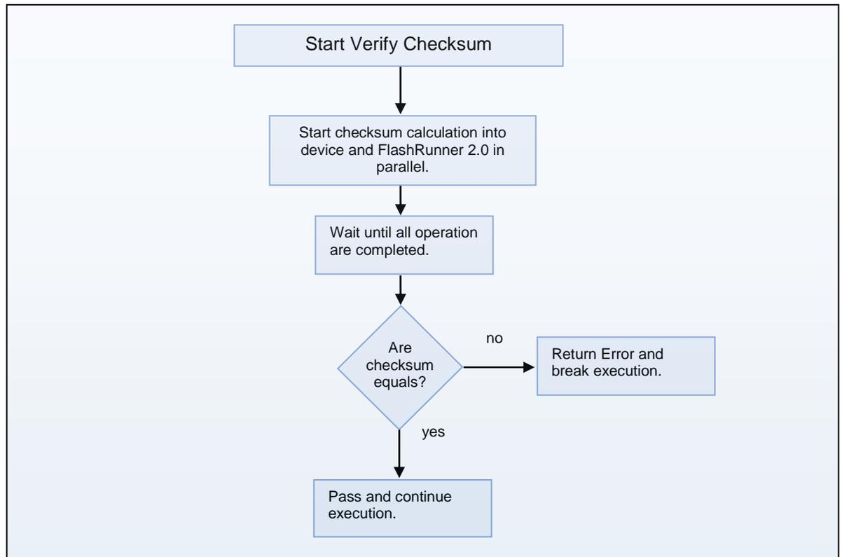
Verify Checksum is broadly implemented in our drivers but some cases could be un-useful. Checksum require a CPU which actually does the calculation, so memories are automatically excluded. Doing target calculation from bare FlashRunner 2.0 read would lead to the same execution time as Verify Readout method.
