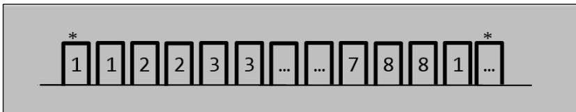
Sampling sequence for 8ch of VPROG0, 300uS per sample, only odd channels are monitored:
